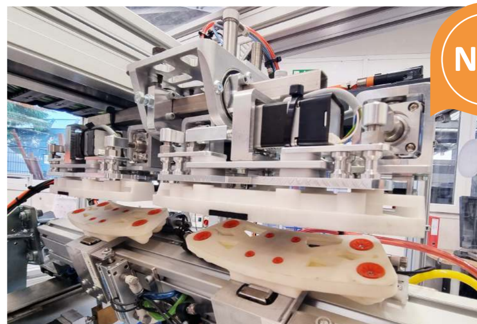
Adjustment heads for even more precise label alignment
