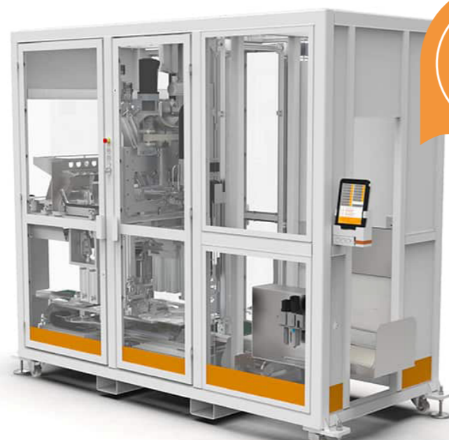
Fully automatic assembly of metal handles on buckets
